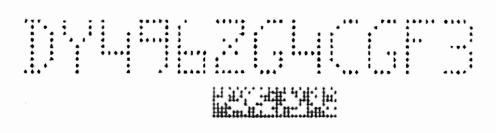
1720 Series optics are designed for 300mm code standards. The high resolution of these wafer readers provide the detail needed for T7 Data Matrix codes, while a large field of view facilitates reading wafer marks such as the SEMI M12 OCR mark shown above.
