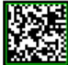
Quiet zone violation
