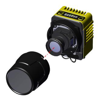
4. Rotate the lens cover into the bayonet mount.
