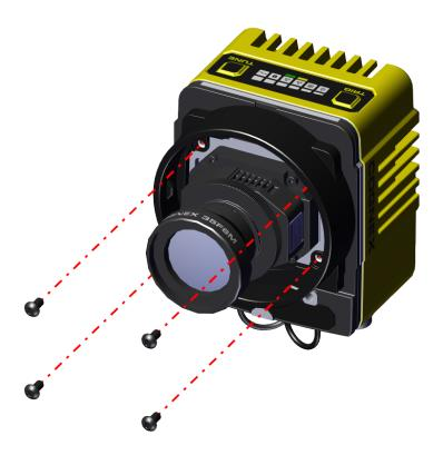
3. Push the lens cover onto the bayonet mount.
