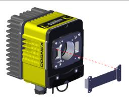
2. Screw in the four screws to attach the lens to the reader.
