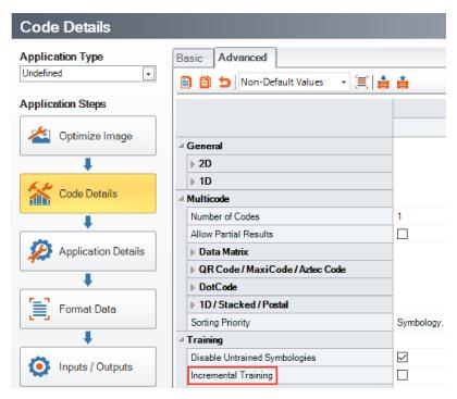
With incremental training enabled, you can train the reader using multiple images showing the symbologies you expect to decode. The reader will train each new symbology while retaining the existing trained symbologies.
