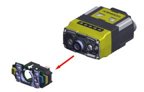
3. Unscrew the two M2x5mm Phillips head screws, remove the 6.2 mm lens mount and the 6.2 mm lens.
