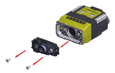
4. Attach the 16 mm lens mount and lens, and screw in the two M2x5mm Phillips head screws. Focus, if necessary. For more information, see <u>Setting Focus</u> on page 57.
