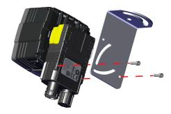
Align the holes on the mounting surface with the mounting holes on the reader. With the reader in right-angle position, only the back mounting holes can be used. To mount the device in right-angle position, use the M3X9 screws.
