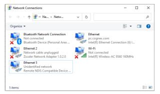
6. Right-click on the virtual adapter and select **Properties**. Assign a fixed IP to the network adapter starting with 192.168.111.
