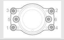
5. Place the lens cover adapter plate on the C-Mount cover, and tighten the screws.
