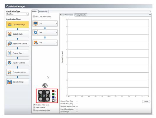
In the **Inputs** / **Outputs** pane, you can assign a LED color for the input/output events. For example, you can set a color for a successful read and set a different color for an unsuccessful read.
