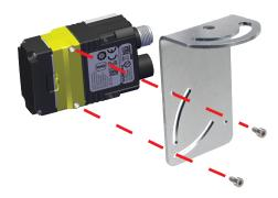
Align the holes on the mounting surface with the mounting holes on the reader. Insert the M3X5 screws into the mounting holes.
