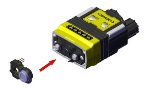
$6. \ \ \, \text{Press the liquid lens onto the imager lens until you reach the stop}.$
