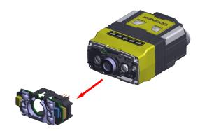
$3. \quad \text{Unscrew the two M2x5mm Phillips head screws, remove the 6.2 mm lens mount and the 6.2 mm lens.}\\$
